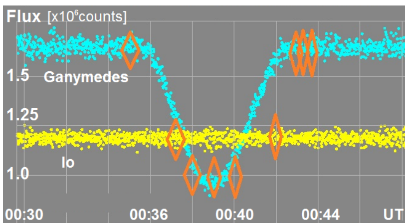
Fig. 1 The light curve of the mutual phenomenon of Ganymede (blue) eclipsed by Io (yellow) on 20 February 2015. Measurements made by Alex Pratt (York); the orange lozenges are the visual observations presented in this paper, in good agreement with the CCD data either in time and magnitude.
